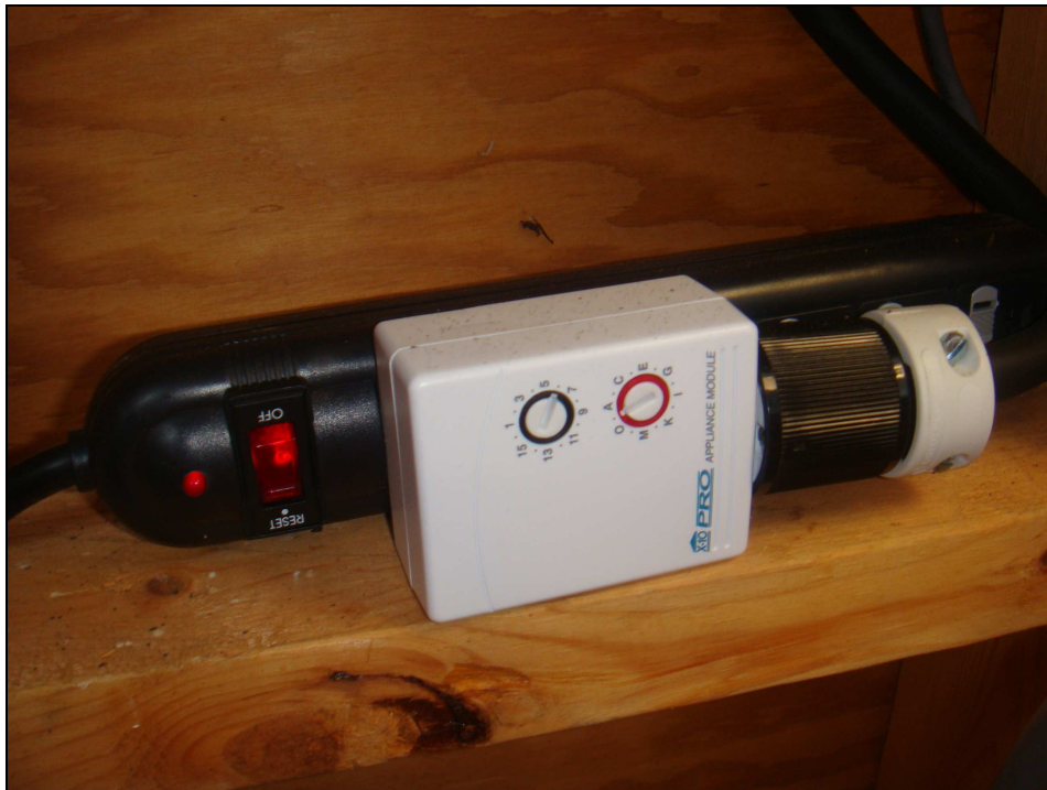
FIG. 69. The X10 module for the dome azimuth control box. X10 allows us to cycle the power to any instrument plugged into an X10 module. (Author)
