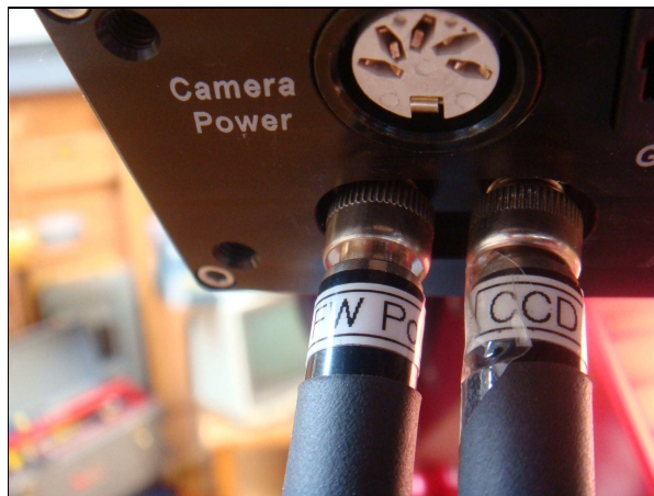
FIG. 17. A close up of the DC power plugs with "locking rings." (Author)
