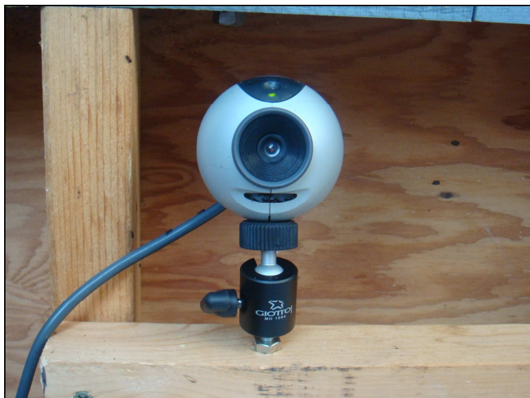
FIG. 67. The webcam mounted inside of the DSO-14 dome allows site managers and Skynet users to check the condition of the dome and telescope. (Author)
