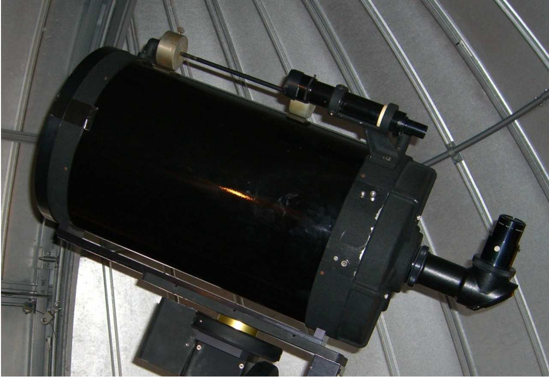
FIG. 18. The C-14 OTA before modification and without instruments attached. (Author)
