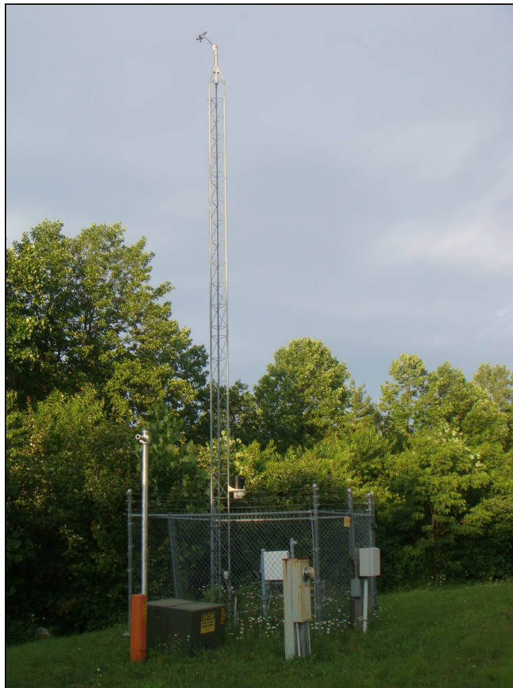
FIG. 71. DSO's Davis Vantage Pro weather station is wirelessly connected to the monitoring computer in the 18-inch telescope's control room. (Author)
