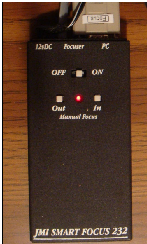
FIG. 51. JMI's Smart Focus controller. The control unit can move the focuser independent from any computer control. However, to use the Smart Focus remotely focus software must connect to the focuser. (Author)
